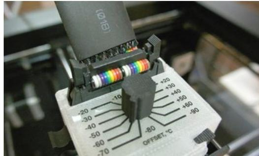
**ANOTHER NOTE:** We've learned that some of the most recent M200s are shipping with ribbon connectors having tabs at the edges of the female connector housing. If these tabs are found to prevent mating with your Z-Temp's male header, simply snip off the tabs with a pair of cutters.
