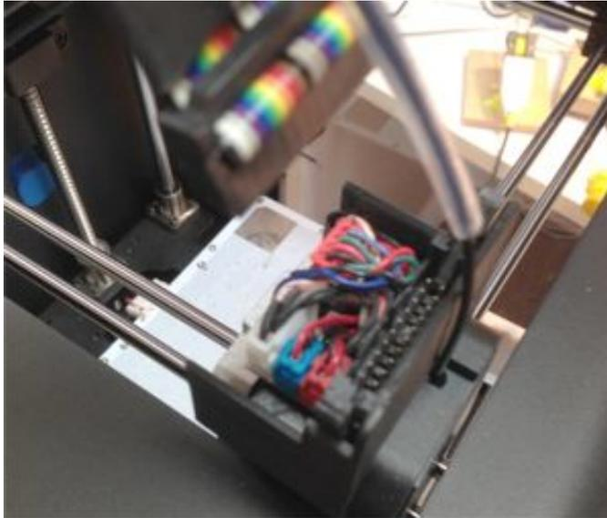
Plug the Z-Temp into the M200's ribbon cable connector, **making sure to line it up correctly.**
